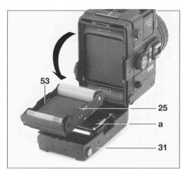
At freezing temperatures (below 0°C) it is better not to preload film inserts; rather load the film directly into the camera and advance to frame No. 1. The adhesive tape holding the film on the backing paper may become brittle in the cold and then cause film-advance problems.
