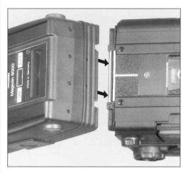
magazine on the camera, at the same time unlocking the metering and exposure functions.
